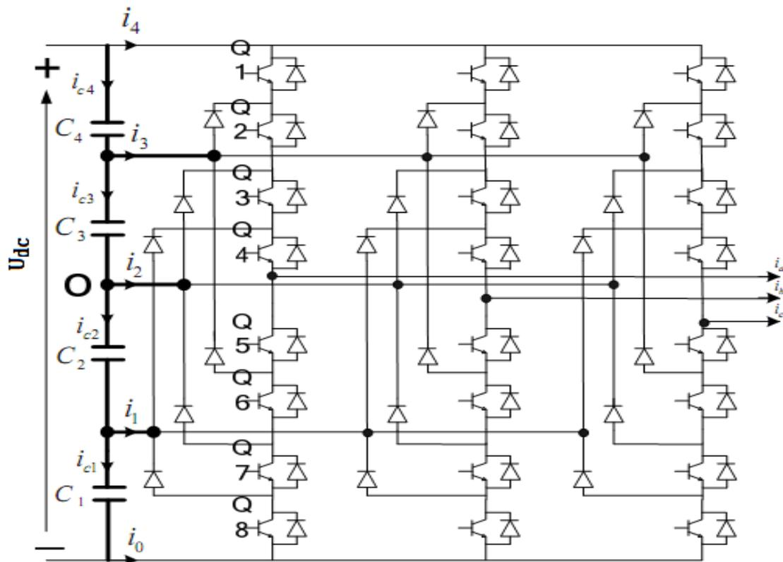
Figure 1. 5L-NPC inverter circuit diagram
