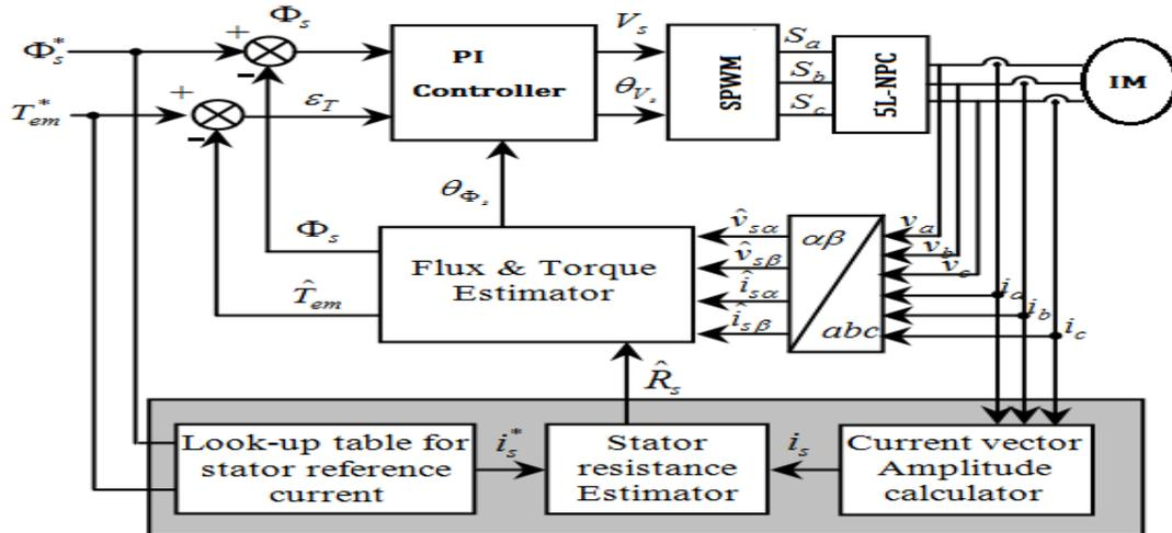
Figure 3. Improved DTFC block diagram with stator resistance estimator
