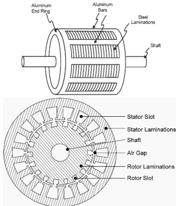
Figure 2. Stator and rotor lamination
