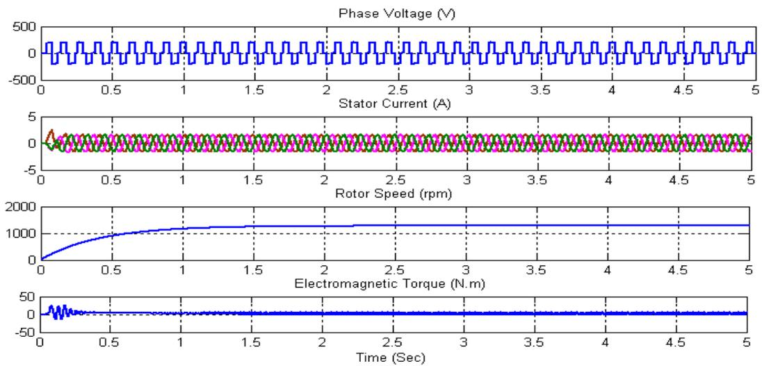
Figure 14. DTC based induction motor performance
