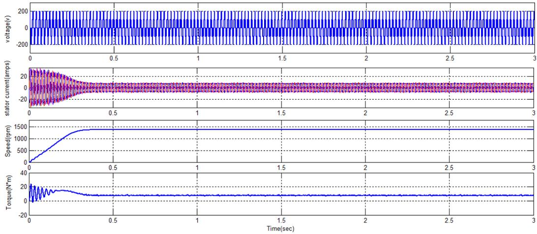
Figure 9. IM drive performance at starting time
