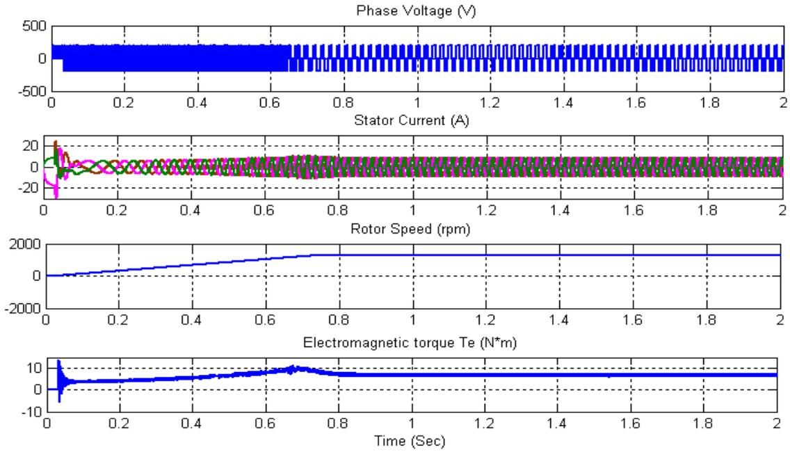
Figure 15. FOC Based induction motor performance
