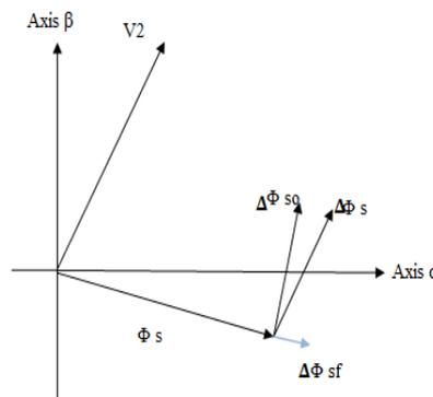
Figure 5. Components of the error of flux at the time of the application of the vector V2 voltage
