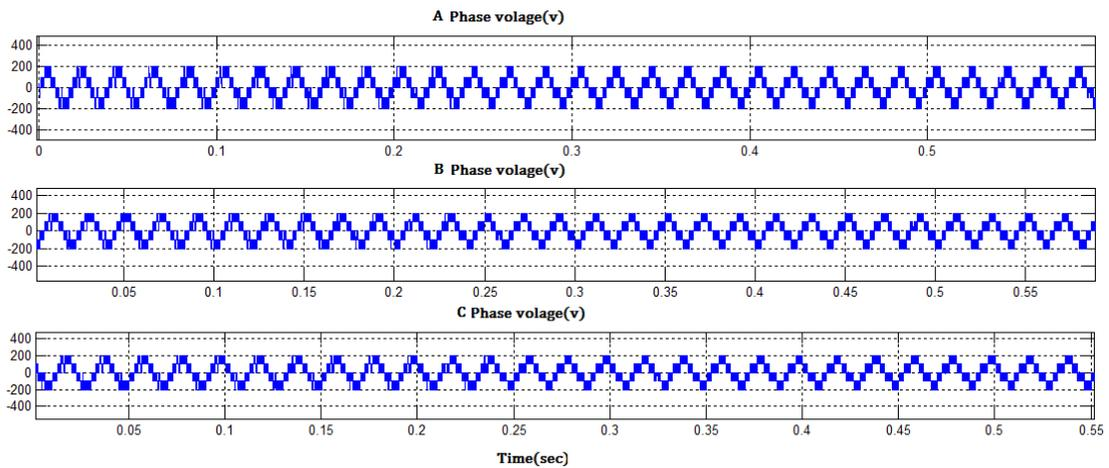
Figure 8. Five Level-NPC inverter voltage
