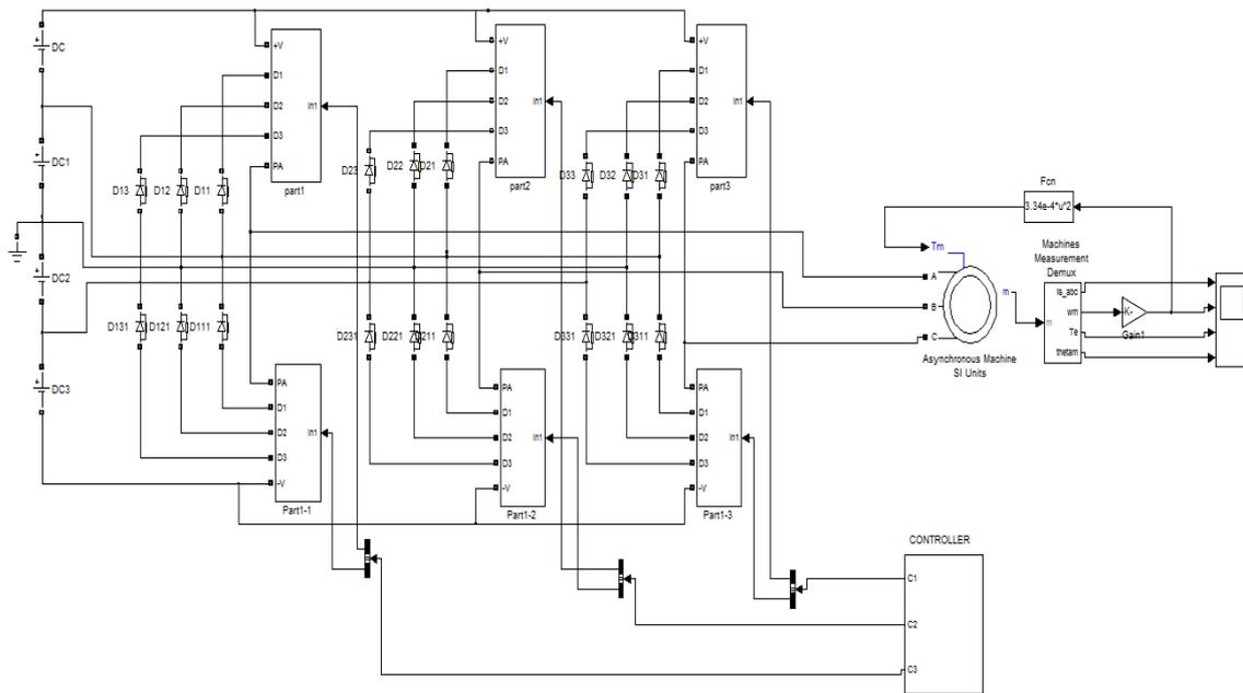
Figure 7. Simulation circuit diagram for NPC-IM
