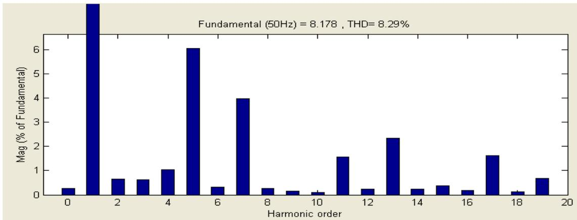
Figure 16. FFT Analysis for proposed topology
