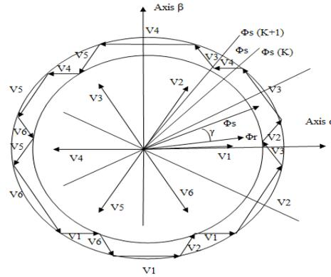
Figure 4. Stator flux increment and spatial positions of the voltage vectors
