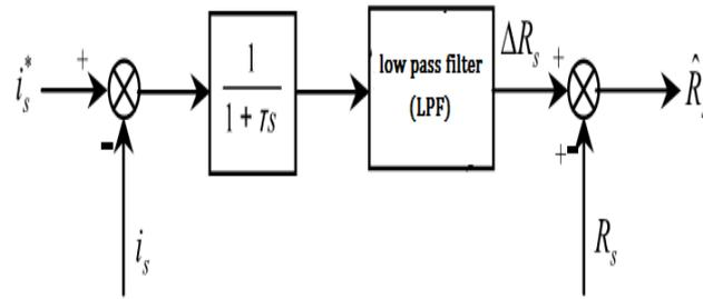
Figure 6. Block diagram of PI resistance estimator
