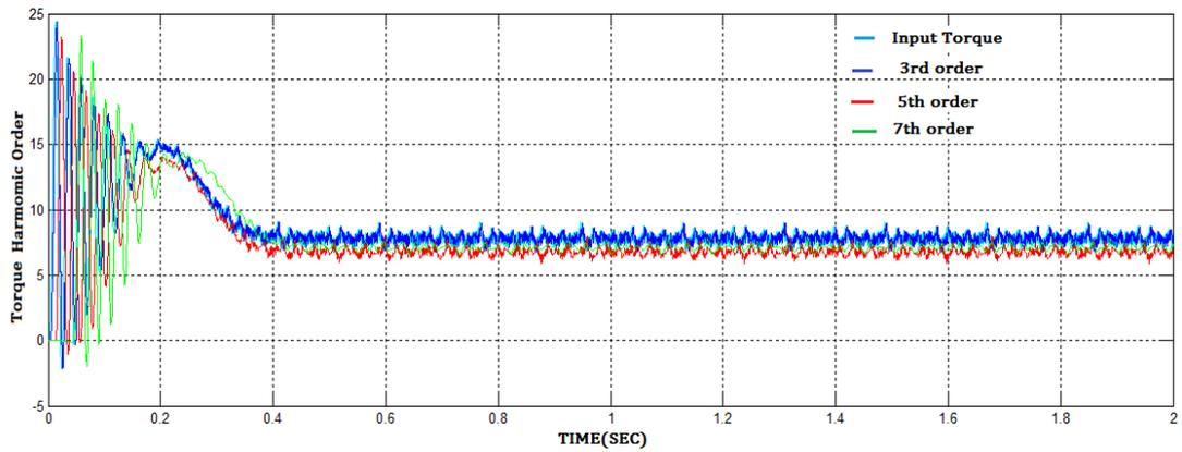
Figure 13. Torque waveforms for different harmonic order
