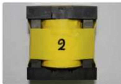
Figure 3. High frequency transformer
