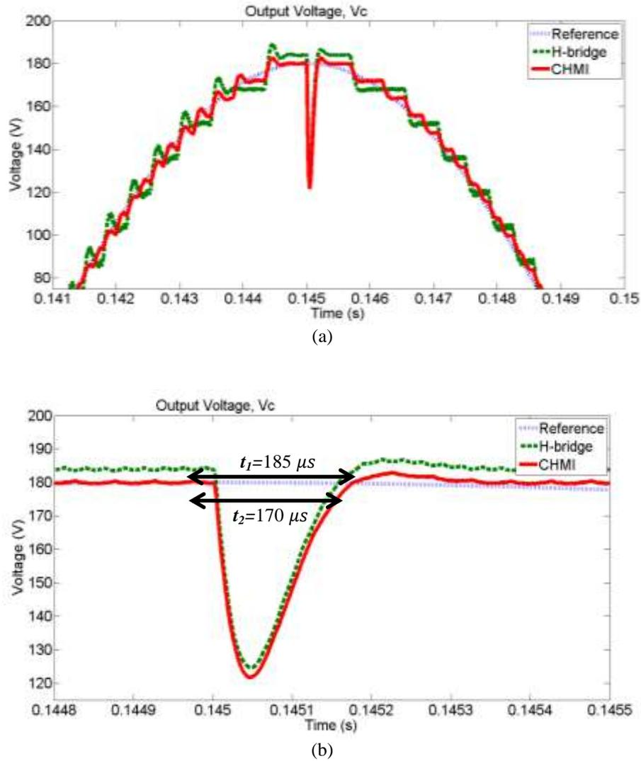
Figure 8. Comparison of output voltage waveform during load uncertainties showing ripples and response time,  $t_1$  and  $t_2$  (a) Ripples (b) Response time
