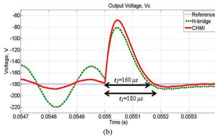
Figure 6. Comparison of output voltage waveform during no load to full load condition showing ripples and transient time,  $t_1$  and  $t_2$  (a) Ripples (b) Transient time
