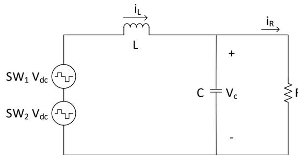
Figure 4. Simplified equivalent average circuit of the 5-level CHMI
