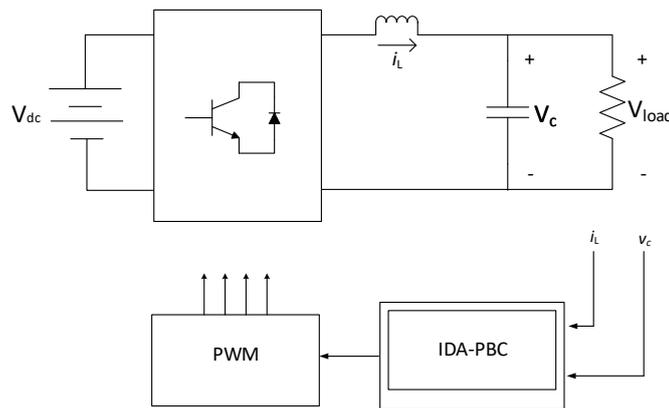
Figure 1. Inverter controlled by the IDA-PBC
