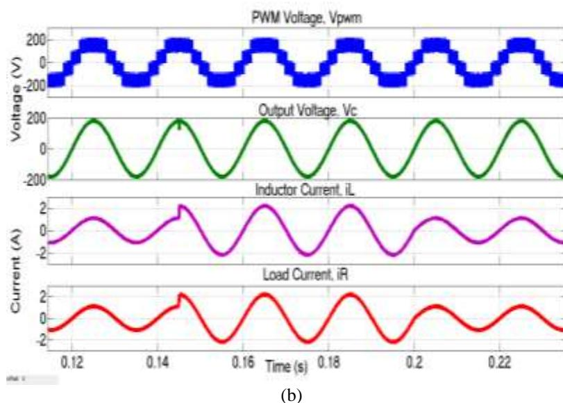
Figure 7. System response under transient operating conditions, top to bottom, PWM voltage  $V_{PWM}$ , output capacitor voltage  $v_C$ , inductor current  $i_L$ , and load current  $i_R$  (a) H-bridge Inverter and (b) 5-level CHMI
