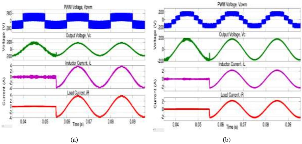
Figure 5. No load to full load condition, top to bottom, PWM voltage  $V_{PWM}$ , output capacitor voltage  $V_C$ , inductor current  $i_L$ , and load current  $i_R$  (a) H-bridge Inverter and (b) 5-level CHMI
