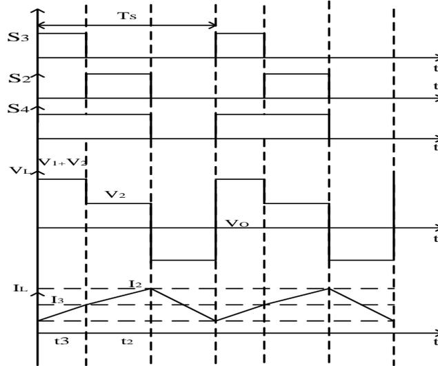
Figure 4. Analytical wave form of the MDIDC converter under buck-boost operation
