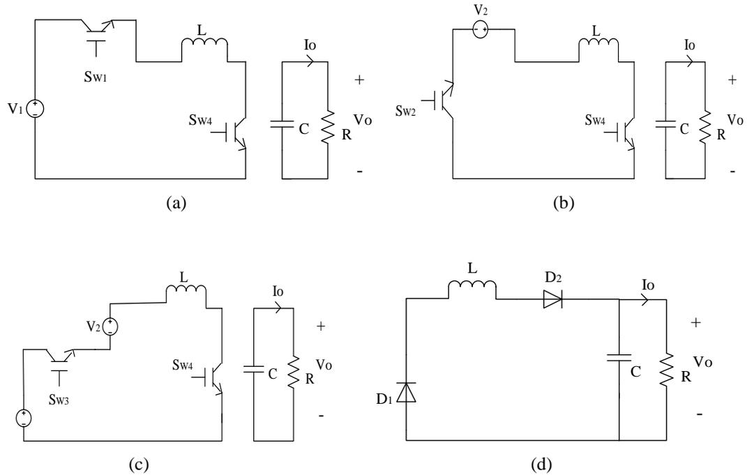
Figure 2. Working states of MDIDC converter: (a) Source  $V_1$  delivers power, (b) source  $V_2$  deliver power, (c) sources  $V_1$  and  $V_2$  together delivers power (d) freewheeling of the output current
