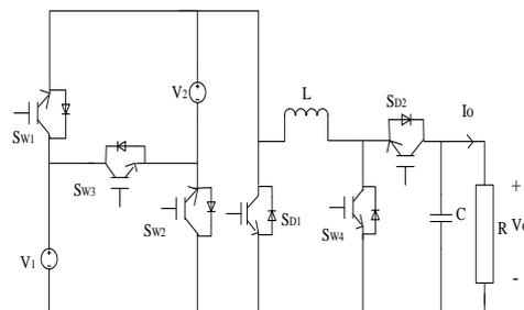
Figure 1. Basic structure of MDIDC converter
