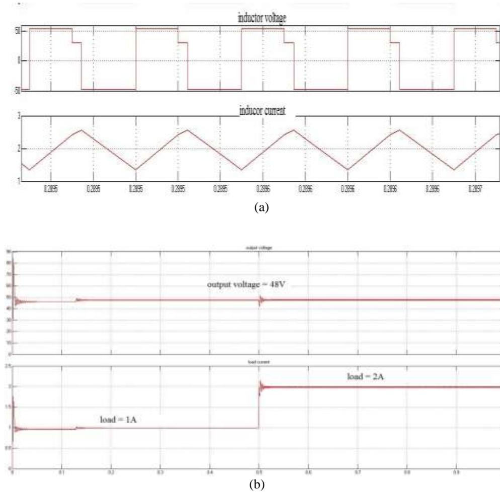
Figure 5. Simulation waveforms of the MDIDC converter under buck-boost operation (a) Inductor voltage and current (b) Output voltage and current under varying load conditions
