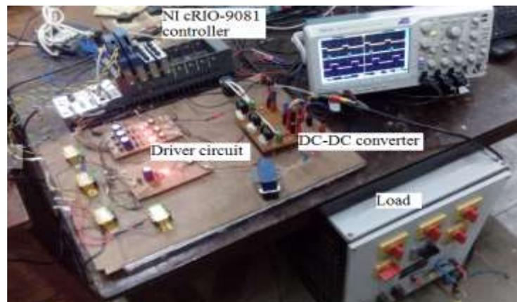
Figure 7. Experimental setup of MDIDC converter with controller
