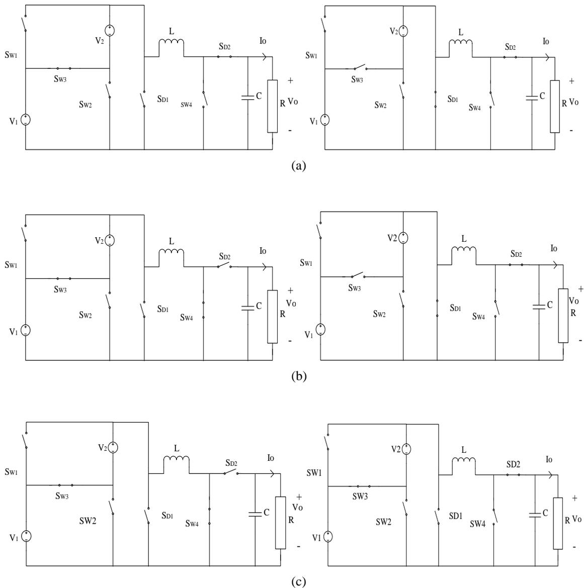
Figure 3. The MDIDC converter under different modes of operation: (a) buck operation, (b) buck-boost operation and (c) boost operation
