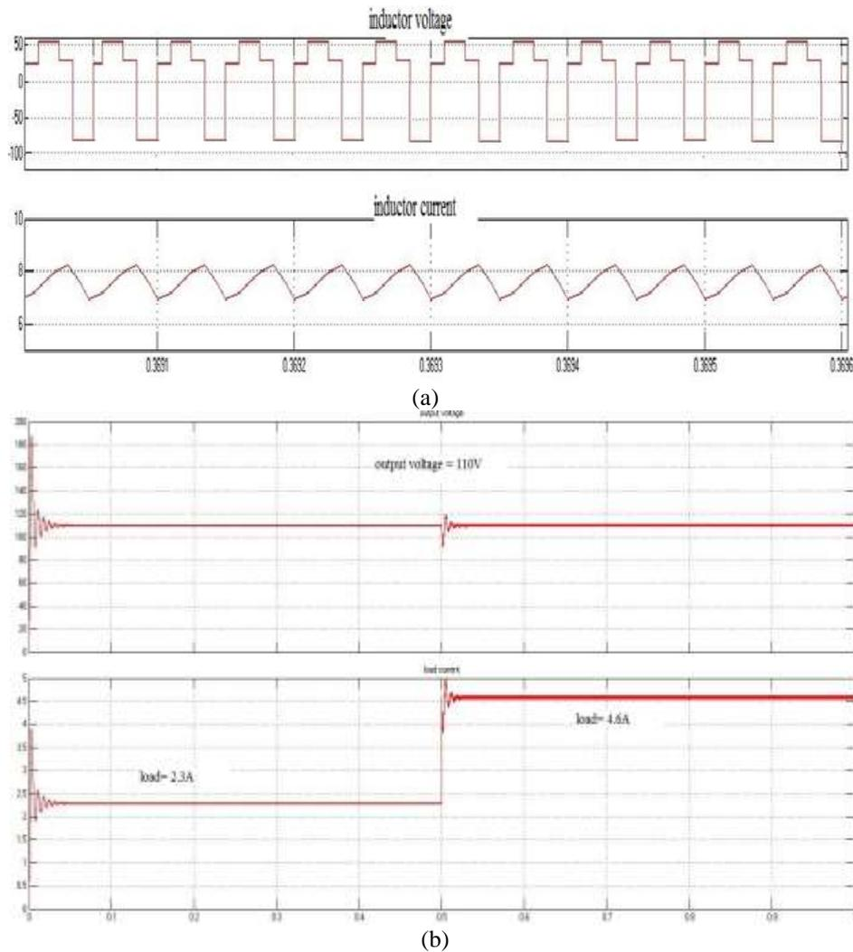
Figure 6. Simulation waveforms of the MDIDC converter under boost operation (a) Inductor voltage and current (b) Output voltage and current under varying load conditions
