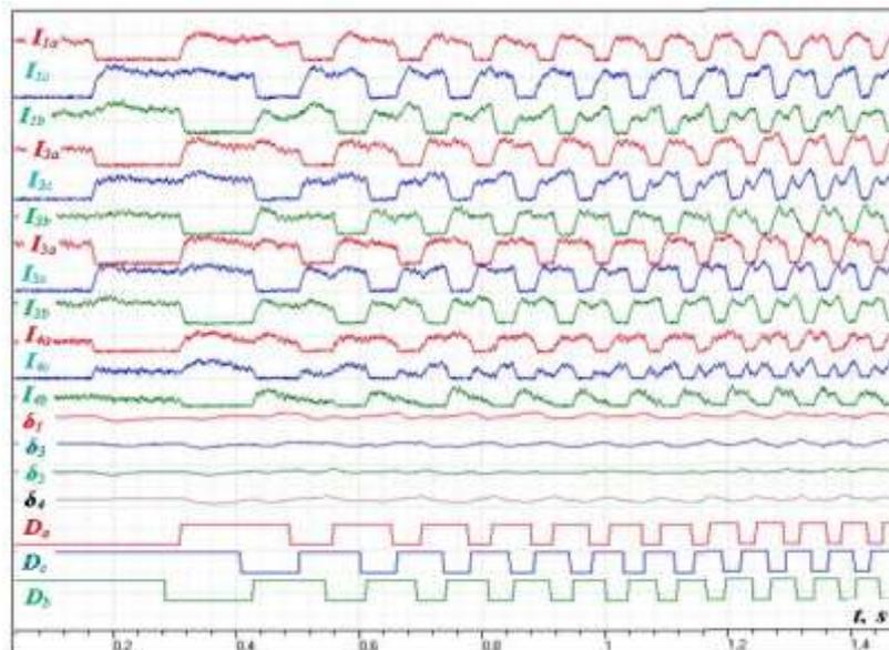
Figure 6. Oscillograms of phase current  $I$ , air gap  $\delta$ , and logic signal  $D$  of position sensors
