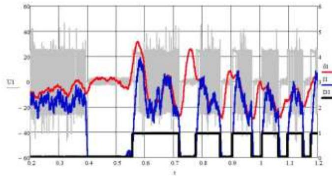
Figure 7. Oscillograms of phase voltage  $U1$ , phase current  $I1$ , air gap  $\delta1$ , and logic signal  $D1$  of position sensors
