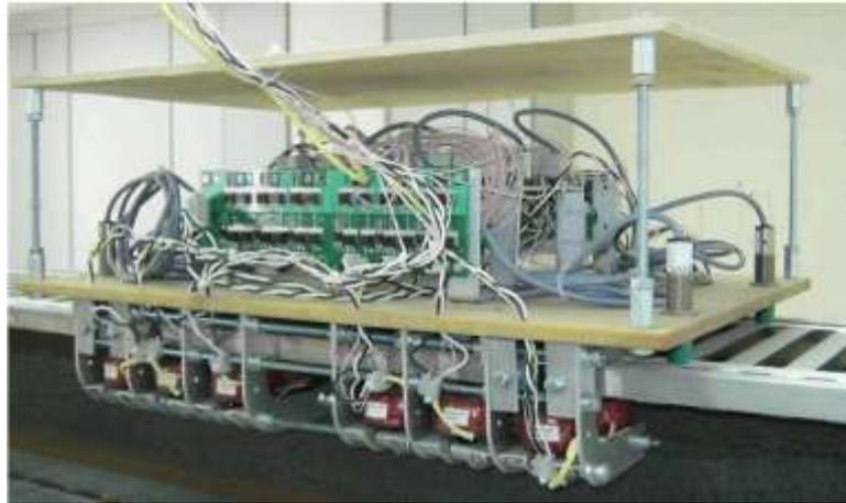
Figure 3. The model of traction levitation vehicle system with magnetic suspension
