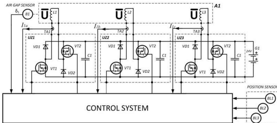
Figure 2. Functional scheme of the combined traction levitation system
