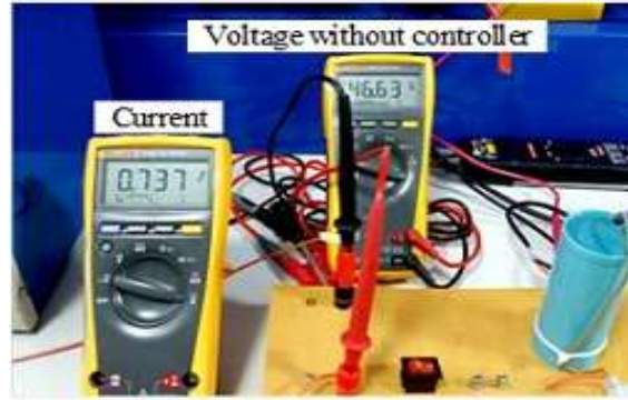
Figure 5c. Experimental output values in rms with resistive loads ( R_1+R_2 )
