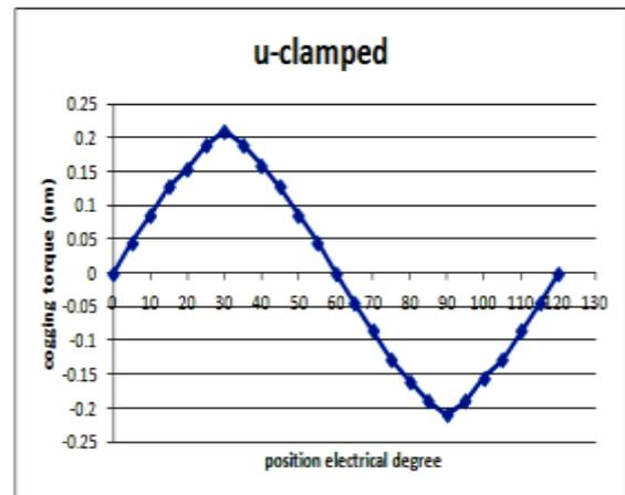
Figure 7. Cogging torque for 8-pole, 60 slot
