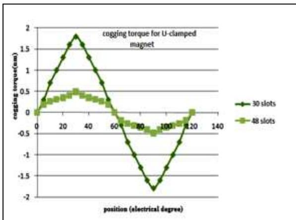
Figure 6. Cogging torque for 30 and 48 slots
