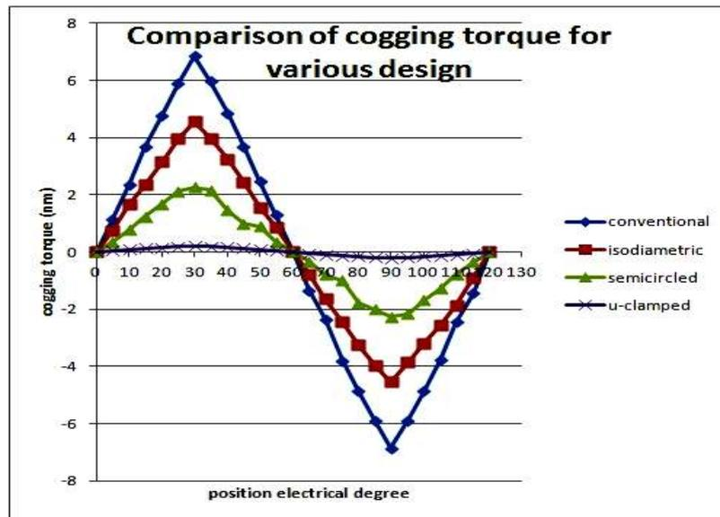
Figure 8. Comparison of Cogging Torque for different model
