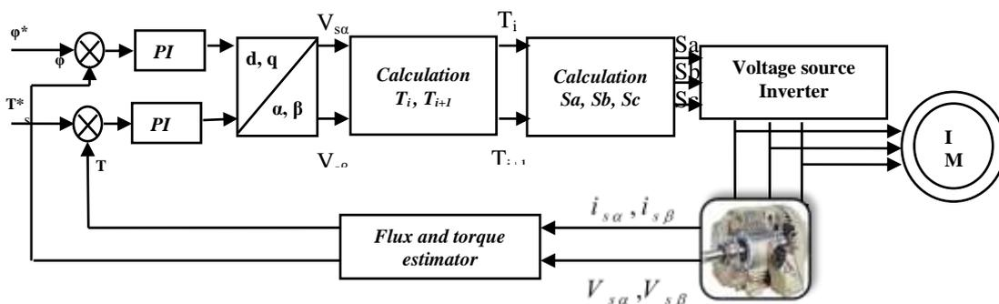
Figure 2. Bloc diagram of DTC
