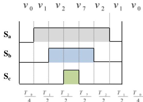
Figure. 3 Sequences of the switches states in sector N1
