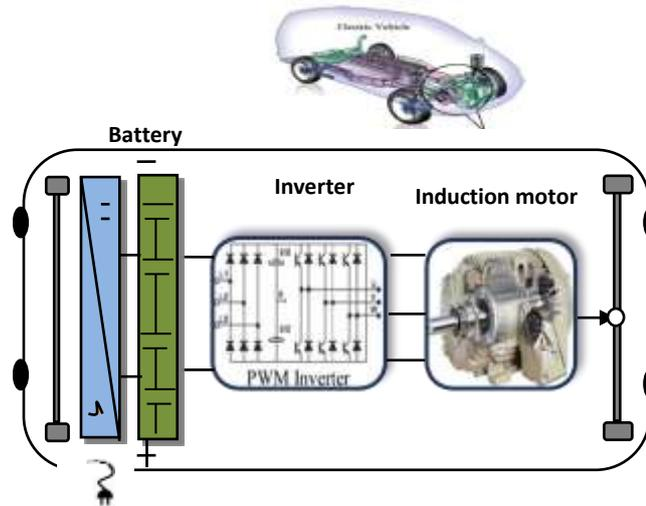
Figure 1. Main components of an EV traction drive.
