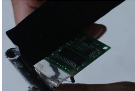
Figure 4. CMPS03 sensor mounted on the tail flipper of anemometer
