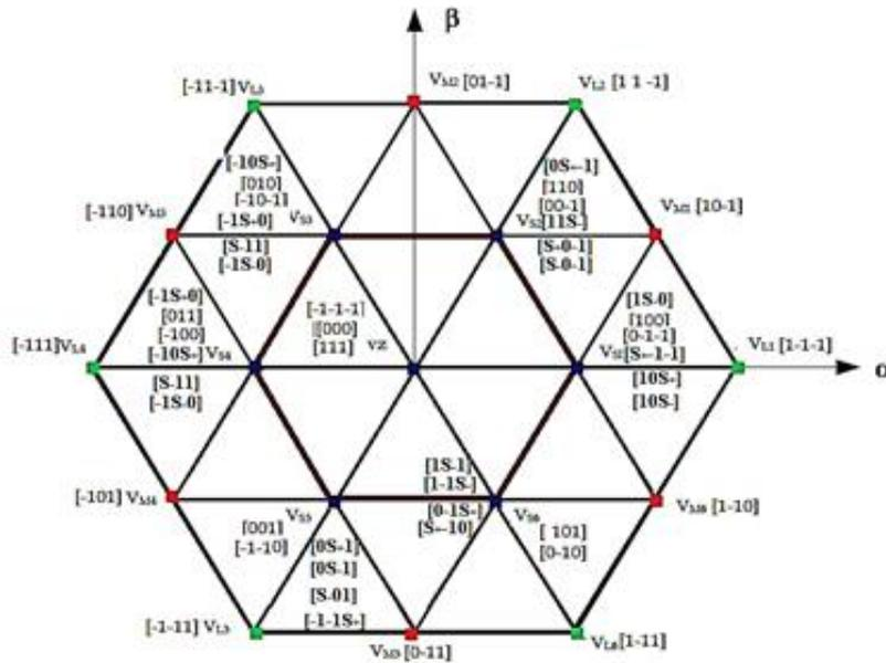
Figure 4. Space vector diagram for the proposed technique
