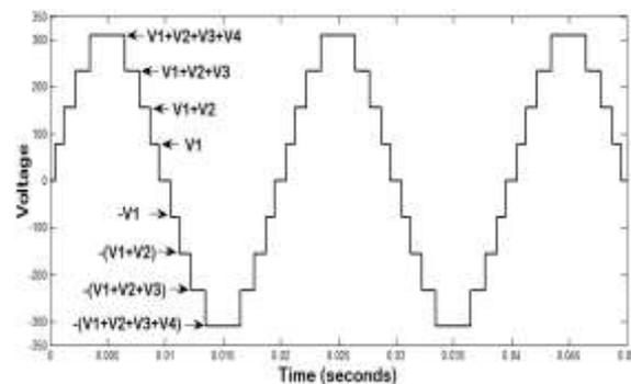
Figure 5. Output wave form of a proposed Multilevel Inverter
