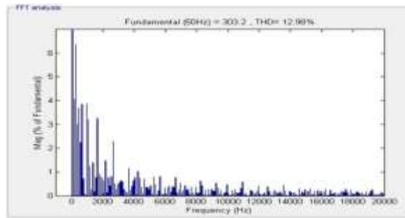
Figure 6. Spectral density of harmonics without modulation
