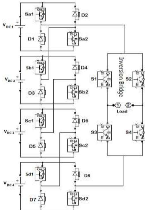
Figure 4. Proposed nine levels Multilevel Inverter
