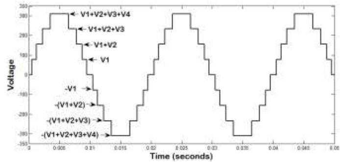
Figure 3. Nine Levels of Classical Cascaded H-bridge Topology
