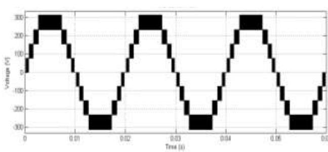
Figure 7. Modulated output of the proposed inverter output
