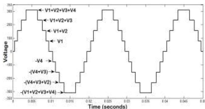
Figure 11. Output with equal voltage source sharing
