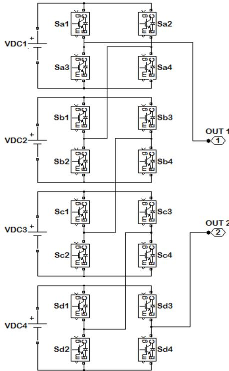
Figure 2. Classical H-Bridge MLI Circuit
