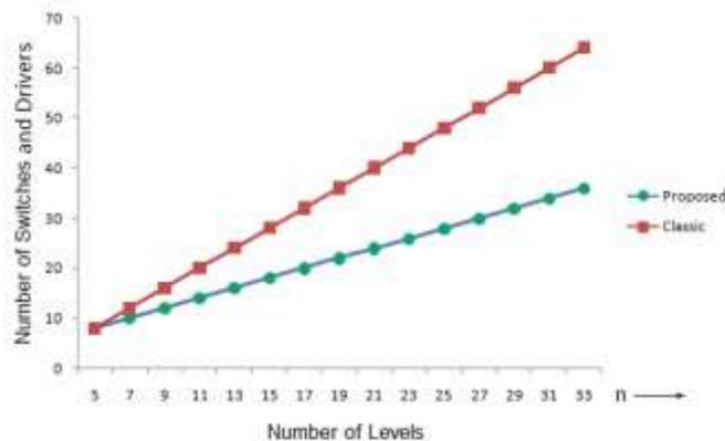
Figure 13. Comparison of the Switches in CHB and Proposed Inverter
