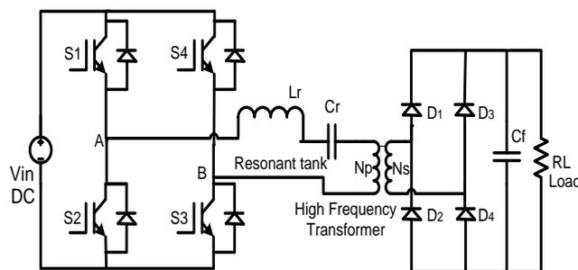
Figure 5. The configuration of the (SRC) with series connected transformer
