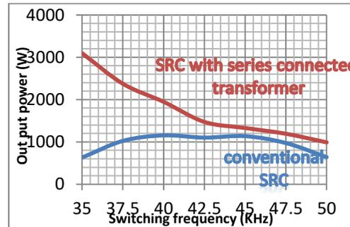
Figure 14. Measured converte output power at different switching frequencies
