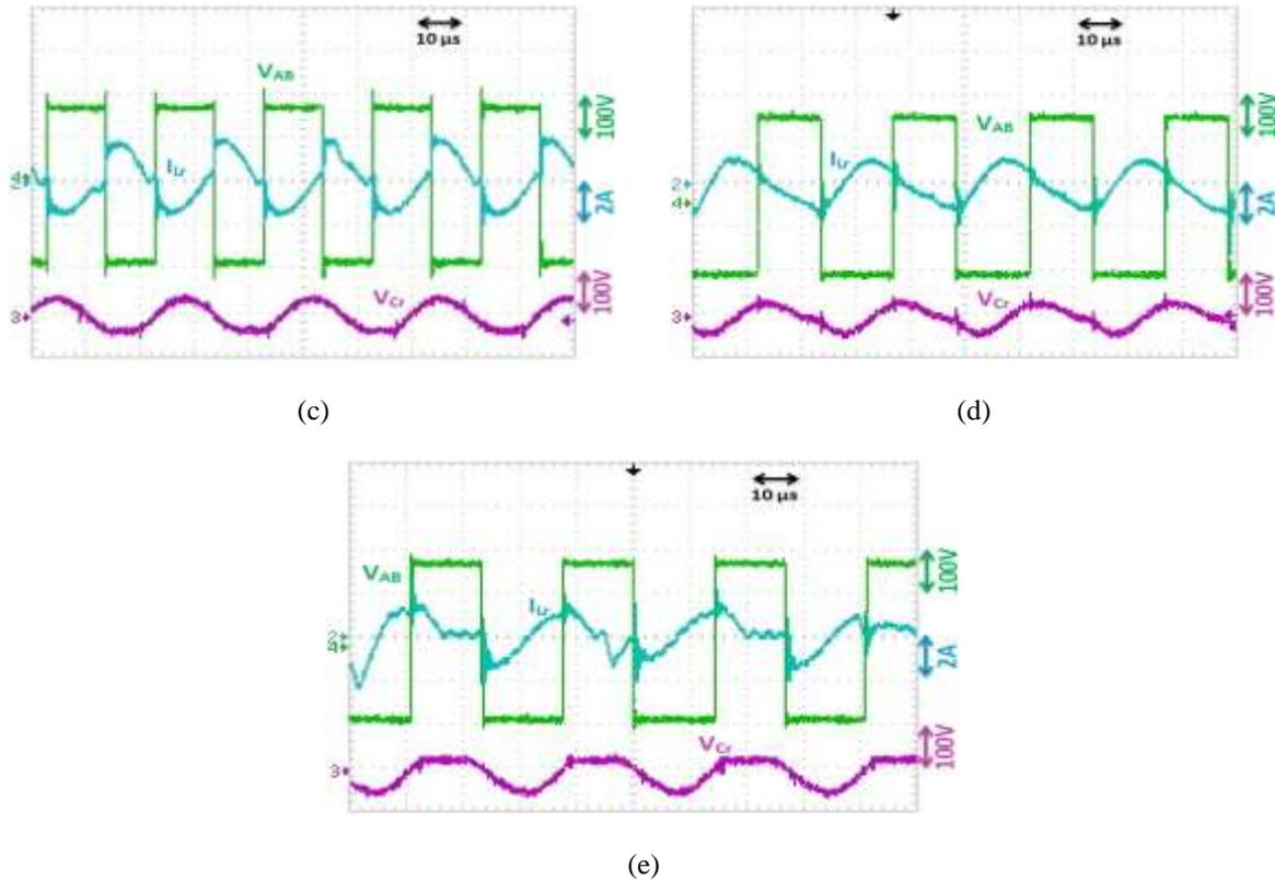
Figure 9. Measured waveforms of the resonant tank input voltage  $V_{AB}$ , resonant inductor current  $i_{Lr}$  and resonant capacitor voltage  $V_{Cr}$  of conventional SRC at  $V_{in}=180$  and (c)  $f_s=42.5\text{kHz}$ , (d)  $f_s=40\text{ kHz}$ , and (e)  $f_s=37.5\text{ kHz}$ .
