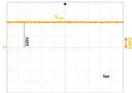
Figure 13. Measured waveform of the output
