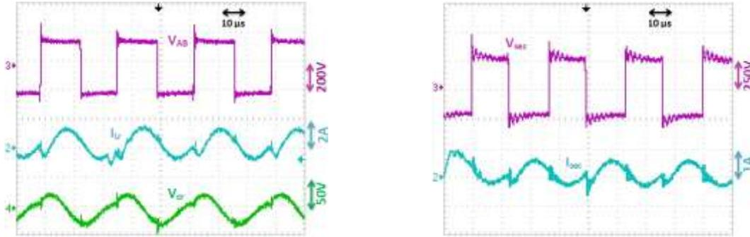
Figure 11. Measured results of the SRC with series connected transformer with  $V_{in}=180$ ,  $f_s=37.5$  kHz and  $Q=2.4$  (a) resonant tank waveforms; resonant tank input voltage  $V_{AB}$ , resonant inductor current  $i_{Lr}$  and resonant capacitor voltage  $V_{cr}$ . (b) the secondary side voltage and current waveforms.
