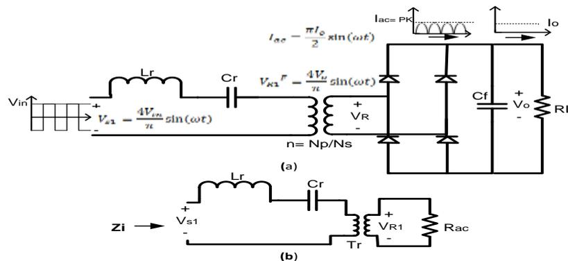
Figure 6. a) The stages and the variables of the converter topology. b) AC equivalent circuit with series connected transformer
