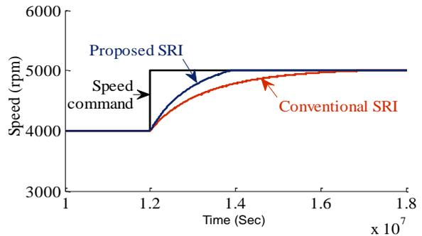
Figure 11. Step speed response.
