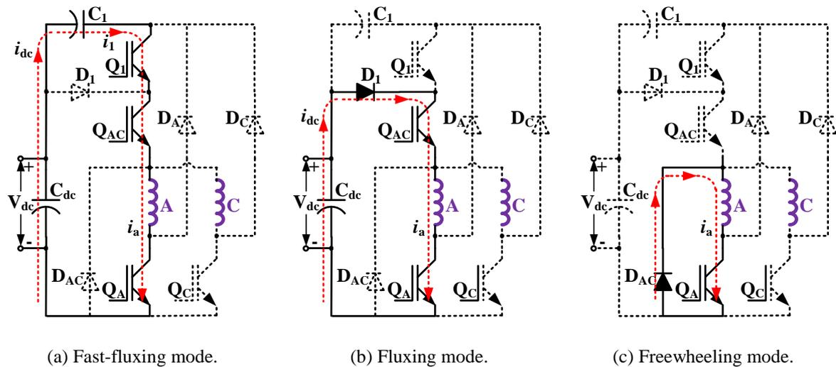
Figure 5. Operating modes of proposed four-phase SRI.
