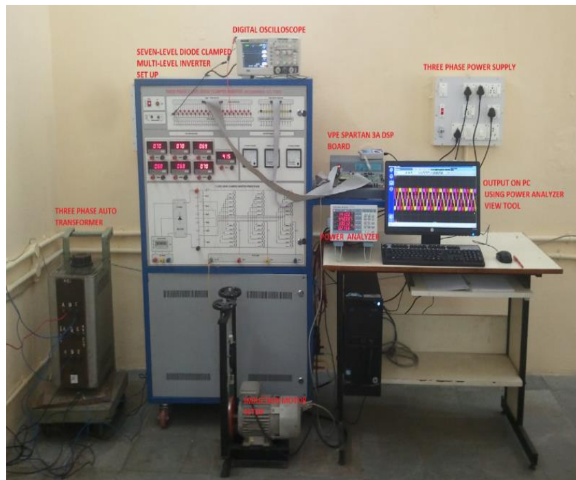
Figure 15. Experimental setup for seven level diode clamped MLI fed IM drive
