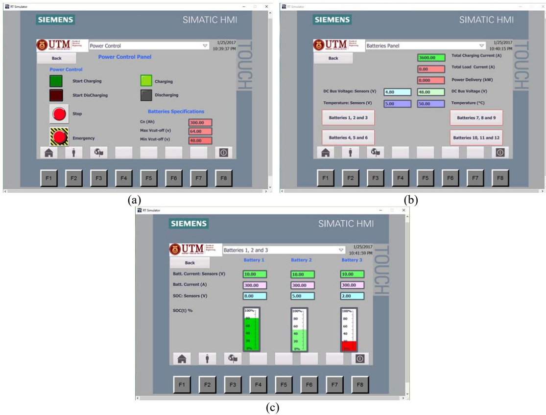
Figure 4. HMI interfaces of (a) Power control, (b) Batteries panel and (c) Batteries 1,2 and 3
