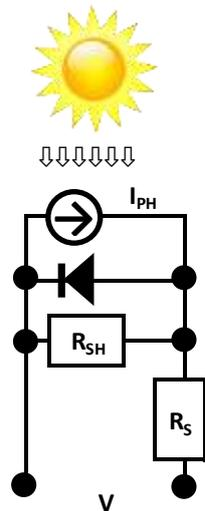
Figure 4. The equivalent circuit of solar cell
