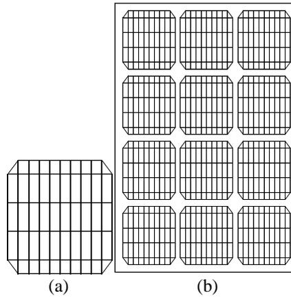
Figure 1. Schematic figure of (a) solar cell (b) solar module
