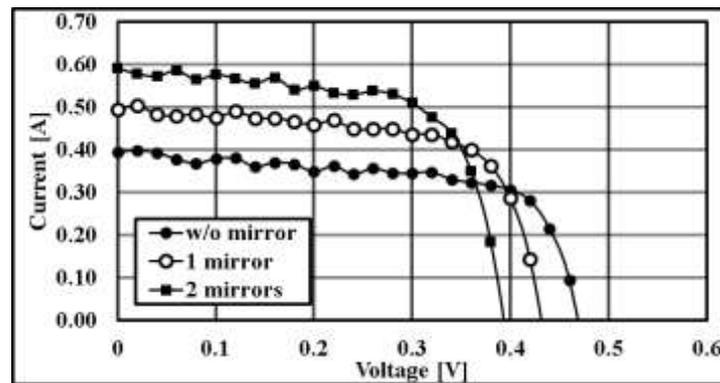
Figure 8. The I-V curve of solar cell with mirror and without cooling
