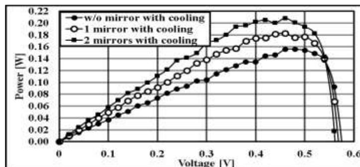
Figure 11. The P-V curve of solar cell with mirror and cooling
