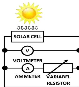
Figure 3. The measurement of solar cell
