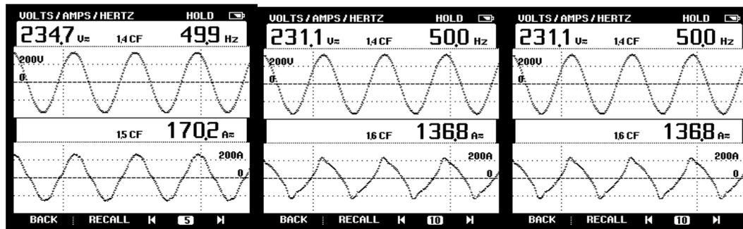
Figure 2. Voltage and current waveform for RYB phases
