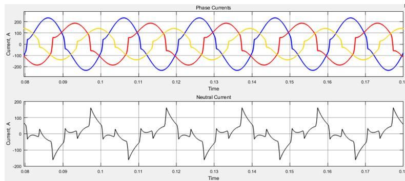
Figure 4. Simulation mode source and neutral current waveforms
