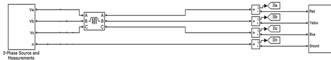
Figure 3. MATLAB simulation model of QUCEST campus
