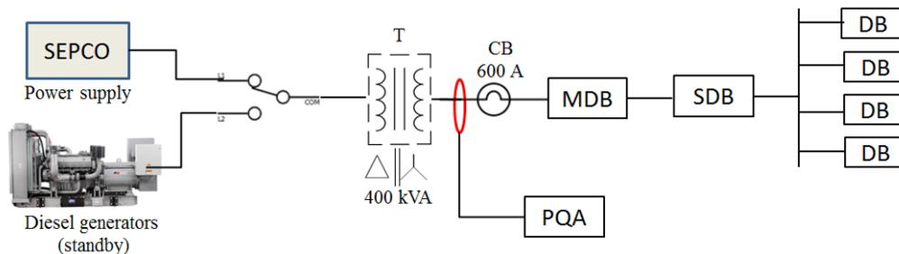
Figure 1. Block Diagram of the Testing System
