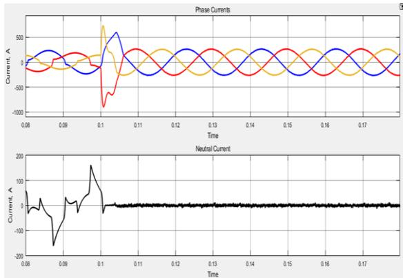
Figure 11. Source and neutral current waveforms for Case 4
