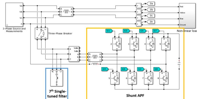
Figure 7. The simulation model of QUCEST campus with the combination of 7<sup>th</sup> single-tuned and shunt APF types of HAPF
