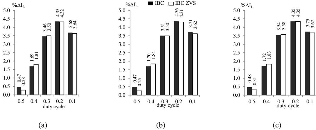
Figure 9. Percentage difference for ripple current  $i_L$  of IBC and IBS ZVS associated with  $V_{out}$  at (a) 48V, (b) 36V, and (c) 24V
