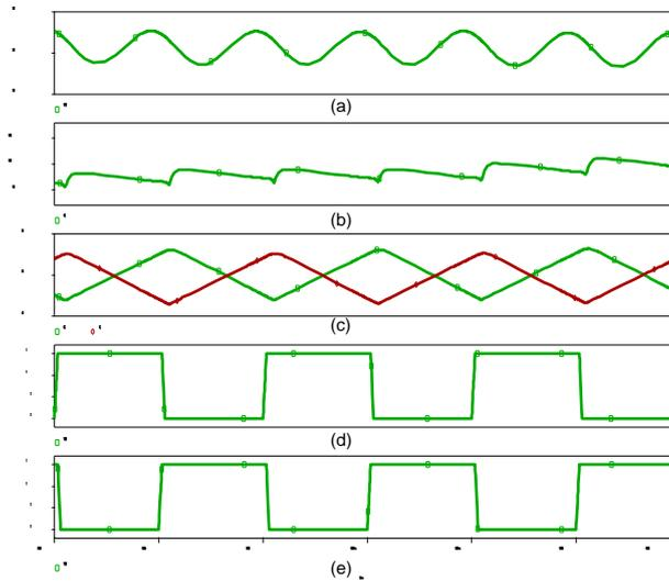
Figure 7. Simulation results for ZVS interleaved dc/dc converter with soft-switching at duty cycle 0.5, (a) ripple output voltage, (b)  $i_L$ , (c)  $i_{L1}$  and  $i_{L2}$ , (d)  $V_{gs1}$  and (e)  $V_{gs2}$
