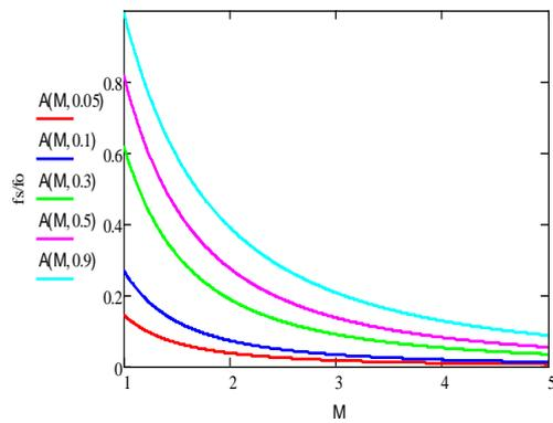
Figure 3. Normalized frequency versus voltage gain;  $n=1$  and  $h \leq 0$
