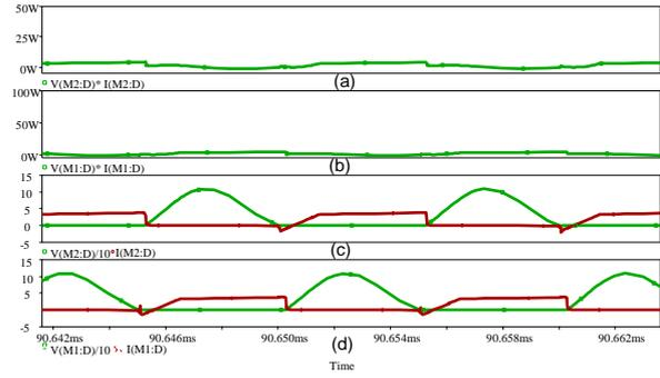
Figure 6. Simulation results for interleaved dc/dc converter with zero-voltage switching at duty cycle 0.5, (a) power loss across  $S_1$ , (b) power loss across  $S_2$ , and (c)  $V_{ds}$  and  $I_{ds}$  across switch  $S_1$  and (d)  $S_2$
