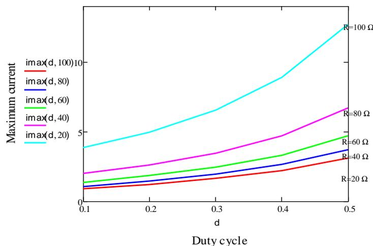
Figure 2. The variation of inductor current  $i_L$  versus duty cycle ( $L=220\mu\text{H}$ ) for single phase boost converter
