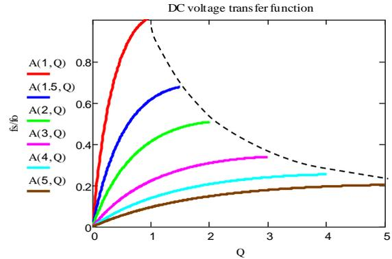
Figure 4. Normalized Frequency Versus Quality Factor;  $N=1$  and  $h \leq 0$
