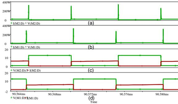
Figure 5. Interleaved dc/dc converter with hard switching at duty cycle 0.5, (a) power loss across  $S_1$ , (b) power loss across  $S_2$  (c)  $V_{ds}$  and  $I_{ds}$  across  $S_1$  and (d)  $S_2$
