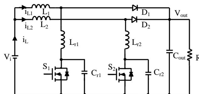
Figure 1. The interleaved dc/dc boost converter with ZVS
