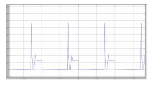
Figure 10. Blocked voltages by switch T<sub>1</sub>
