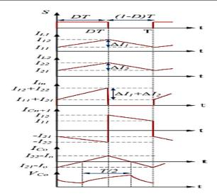
Figure 4. Waveforms of proposed enhanced zeta
